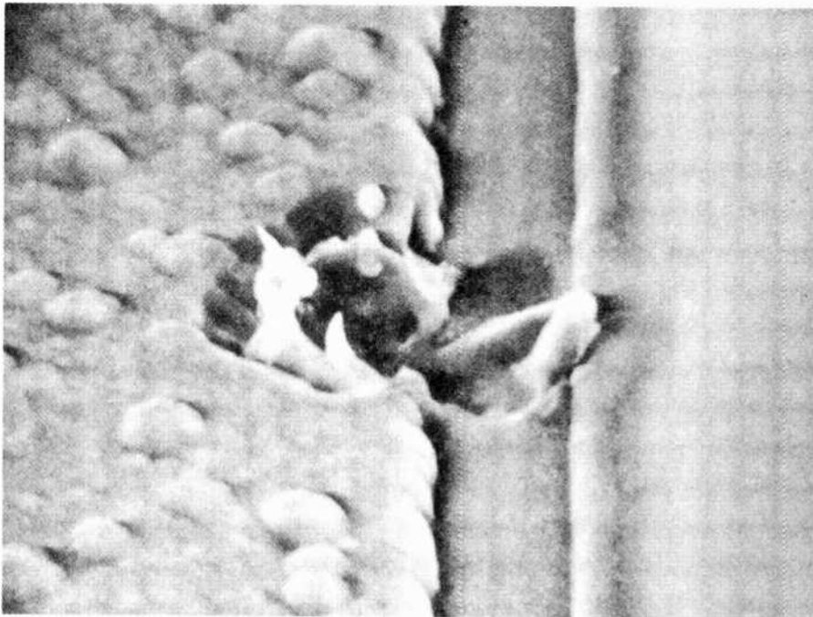
Fig. 2. Magnified (4300X) view of a cell-destroying punchthrough that has catastrophically destroyed the semiconductor device.
